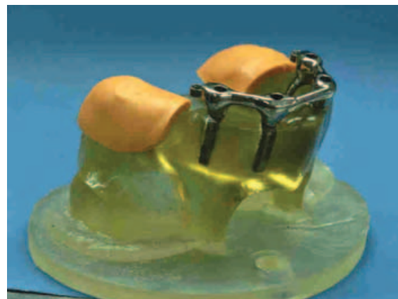
Figure 1. Photoelastic model with splinted bar-ERA attachment system.
