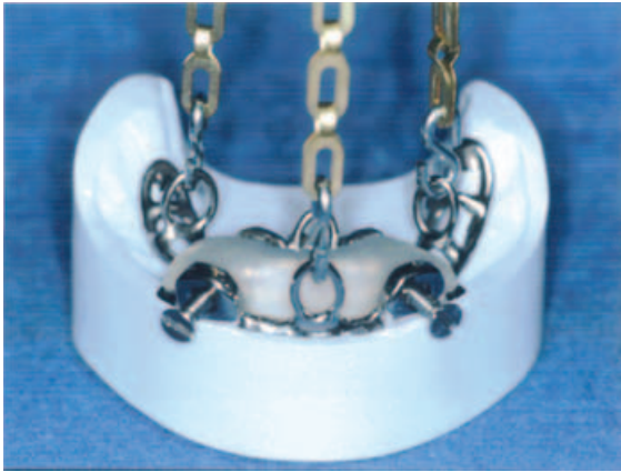
Figure 5. Experimental overdenture assembly connected to the universal testing machine.
