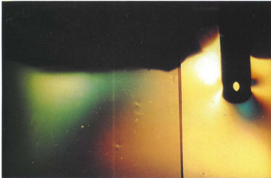
Fig. 12. Load at second molar for model IA (view of loaded side). Models IB and IC exhibited similar characteristics.
